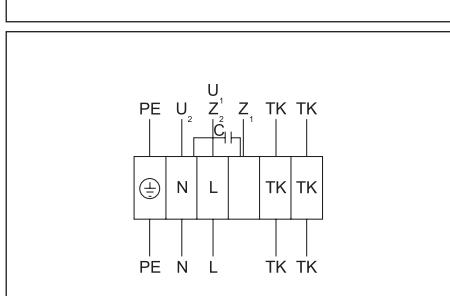
**Wiring diagram No. 4 (1~230V)**
