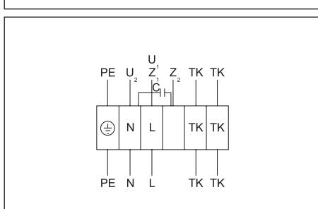
**Wiring diagram No. 3 (1~230V)**
