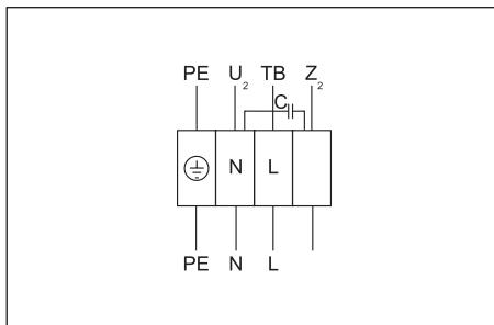
**Wiring diagram No. 1 (1~230V)**
