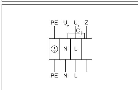
**Wiring diagram No. 2 (1~230V)**
